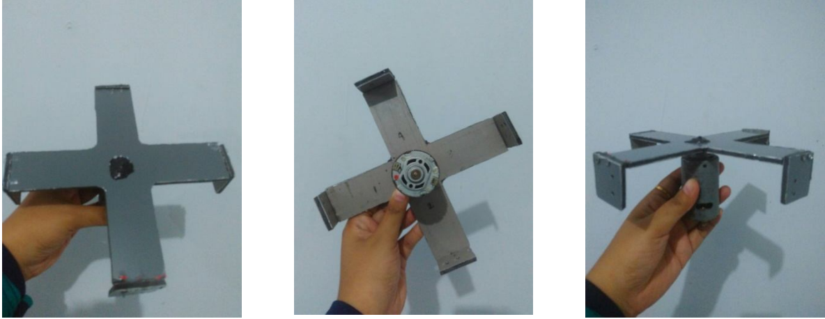
FIGURE 6. Construction of the dynamo and blade base
